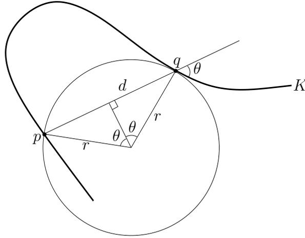
Figure 5.1: In the proof of Lemma 5.2.3, the circle tangent to  $K$  at  $q$  and passing through  $p \in K$  has radius  $r = d/(2 \sin \theta)$  where  $d = |p - q|$  and  $\theta$  is the angle at  $q$  between  $K$  and  $\overrightarrow{pq}$ .
