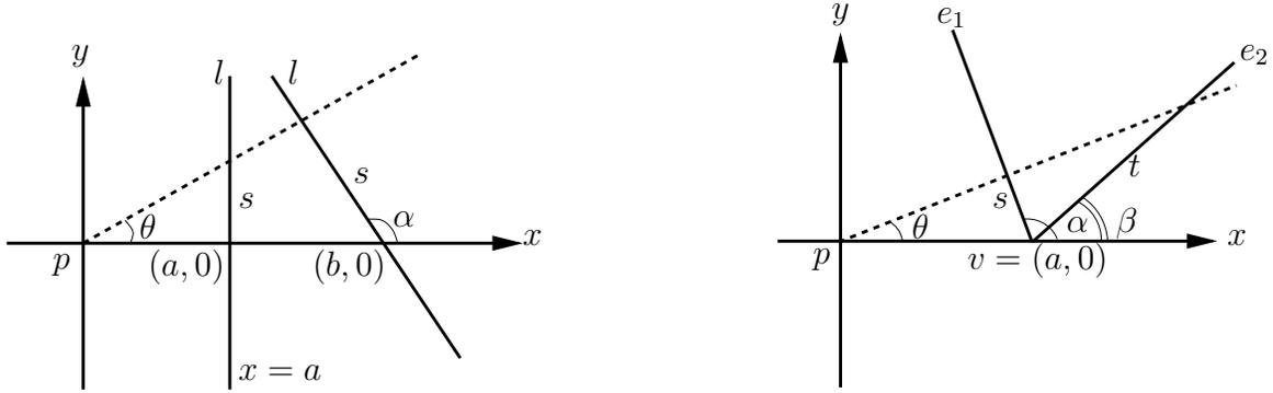
Figure A.1: Left picture shows how arclength  $s$  along a line  $l$  depends on the point of intersection with the  $x$ -axis, the angle  $\alpha$  and the angle  $\theta$ . The right picture shows how we may compare the arclength  $s$  and  $t$  along edges  $e_1$  and  $e_2$  respectively, as we move along the interval of trisecants.
